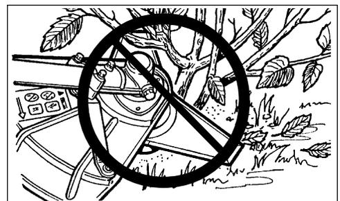
**8 Tooth Weed/Grass Blade P/N 69600120331** is designed for grass, garden debris and thick weeds. **DO NOT** use this blade for brush or heavy woody growth, 3/4" in. (19 mm) diameter or larger.
